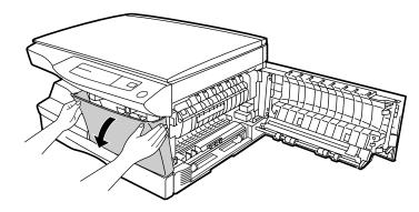
Rotate the feeding roller in the direction of the arrow and gently remove the misfed paper from the exit area.
